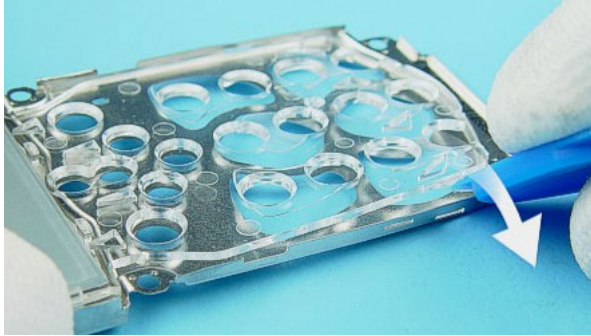
Unlock the LCD snaps of the LCD Light guide on the bottom side.
